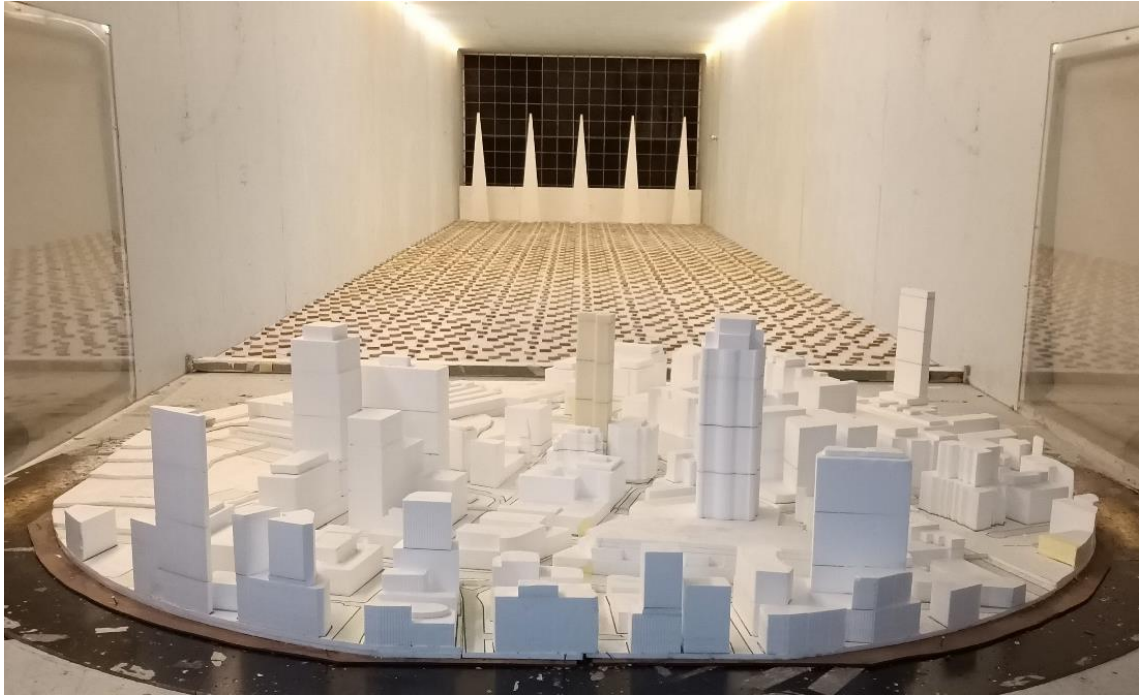
Figure 1c: Close up photograph of the Wind Tunnel Model (Proposed DCP Envelope, view from the north)
